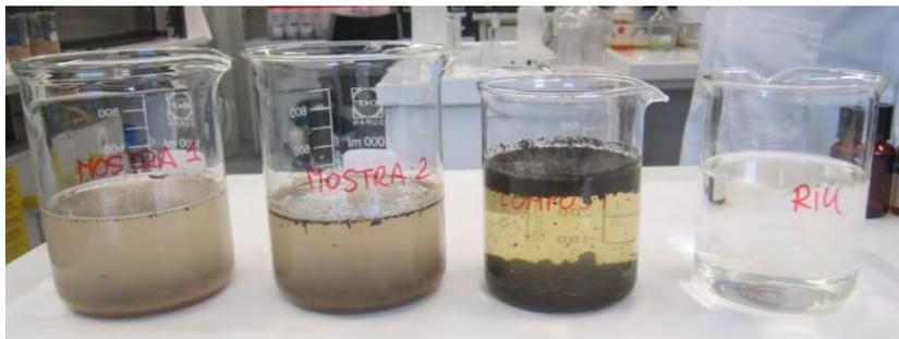
Figure 6-9: Leaching test performance, Above, in the initial shake gently; below after two hours
